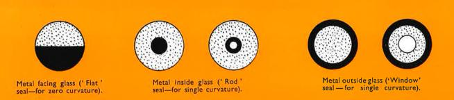
Fig. 2.—Diagram showing the three basic types of seals. (By courtesy of The British Thomson-Houston Co. Ltd.)
