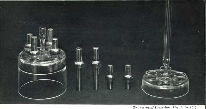
Fig. 9.-Component parts of a large transmitting valve showing Nilo K cups brazed to copper rods.
