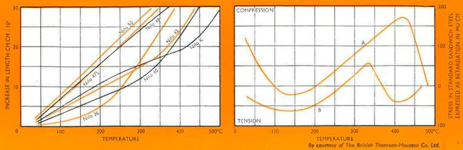
Fig. 7.—The curves on the left show the thermal expansion of the iron-nickel alloys of the Nilo series in the fully annealed condition. On the right are shown the stress—temperature curves for Nilo K with C.40 glass (A) and Nilo 475 with C.12 (B) glass.
